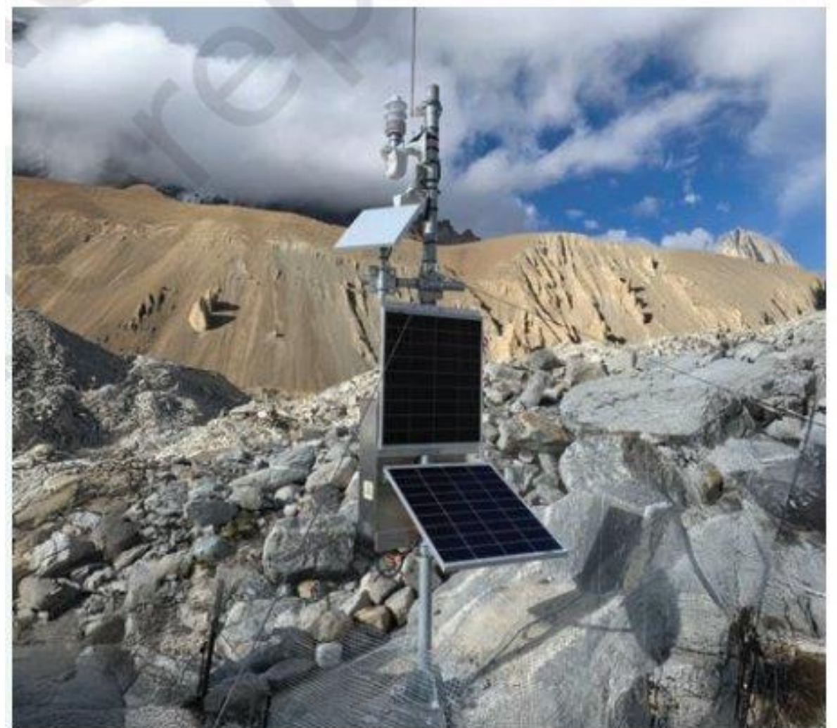
Fig. 2.12. AWS at a glacial lake of Sikkim
